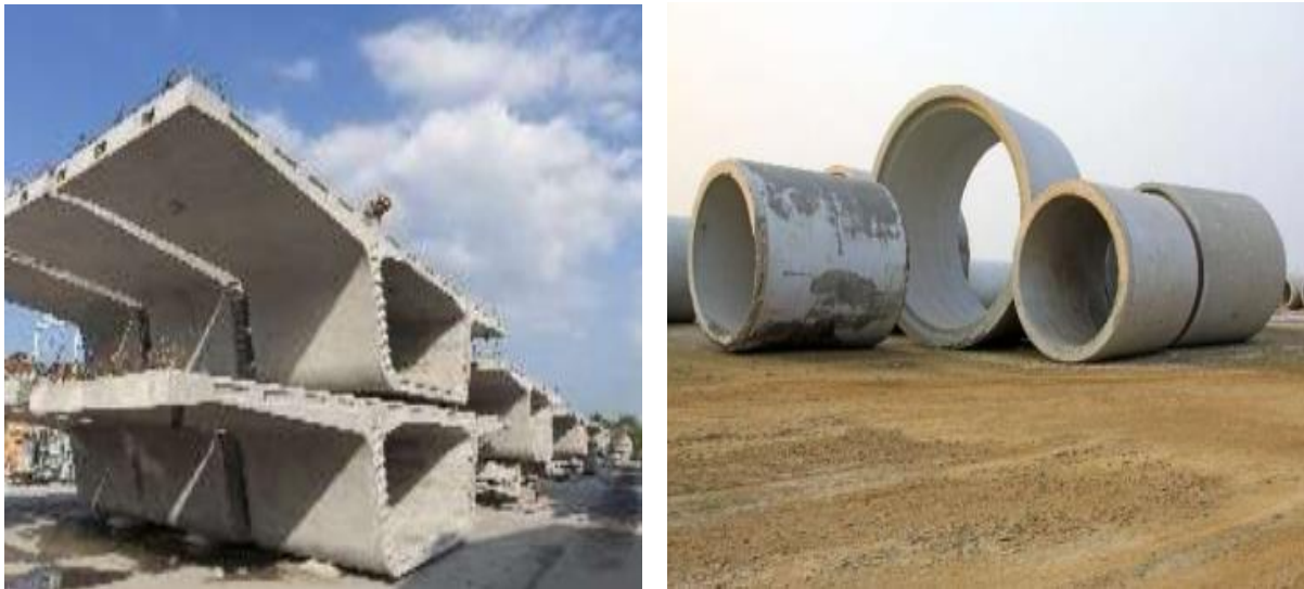
Figure 5. Prefabricated components of bridge and pipe (CIC, 2018b)
